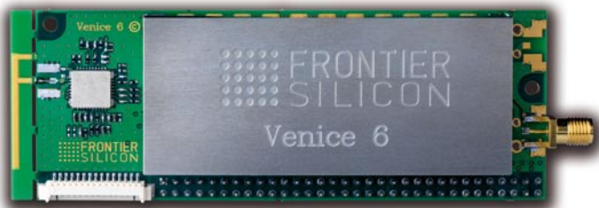
Venice 6 - 45 x 113 mm, including snap-off Wi-Fi PCB antenna (left)
